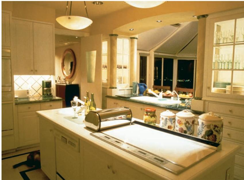
**Plate 7-2 (bottom)** Kitchen, modern transitional, with decorative, task, focal, and ambient layers. Note lighting inside of glass-faced cabinets serves as a focal layer. *Photo: J. Benya*
