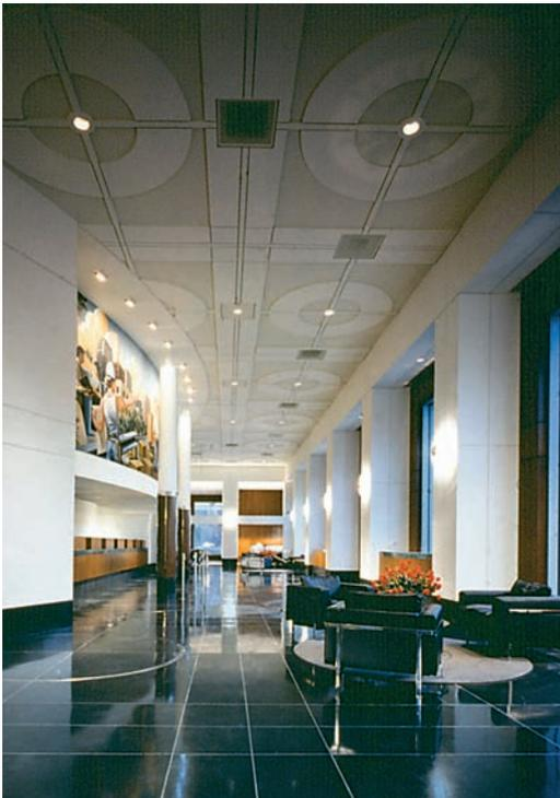
**Plate 8-3 (far left)** Modern Bank. Downlights provide general and task lighting. Wallwashers provide focal lighting for mural over teller line. Ornamental sconces provide decorative and ambient lighting with additional ambient lighting from beams. *Photo: RMW Architects*
