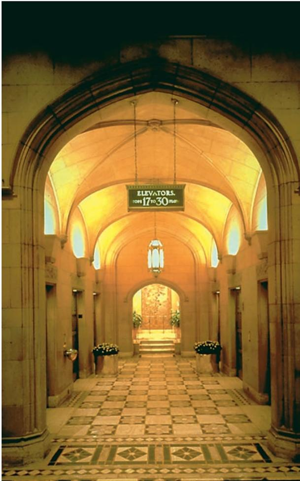
**Plate 5-1** Elevator Lobby, Historic (Gothic-inspired). Chandelier in gothic style is decorative only. Ambient light and illumination of groin vaults by sconce uplights. Task light created by downlight over elevator doors. Focal light on wall at end of hall provided by wallwashing. *Photo: J. Benya*
