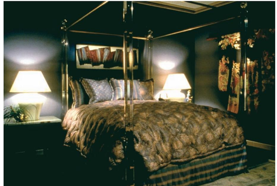
**Plate 7-4 (bottom)** Traditional Bedroom. Decorative lamps provide eye-level glow and ambient light—but reading light is provided by recessed task lights, and focal light is provided by recessed accent lights. *Photo: J. Benya*
